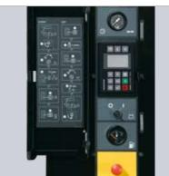
Available for MOBILAIR compressors with free air deliveries up to 26.9 m<sup>3</sup>/min, the innovative 'SIGMA CONTROL mobile' compressor control system is simple to use and precisely matches motor power to actual compressed air demand. This significantly enhances both compressed air availability and fuel efficiency.
